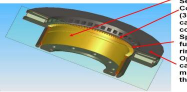
Separate tone ring Cooler temperatures (300 F cooler than cast-in teeth) reduce corrosion. Special coatings further prolong tone ring life. Optimized disc casting and better machining reduce thermal stresses.
