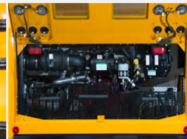
A maintenance shelf allows for quick and easy fluid checks and routine maintenance. The shelf can be easily removed to provide full engine access.
