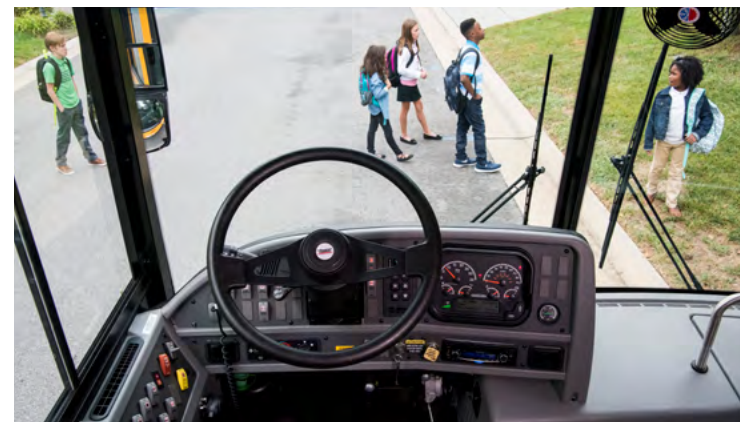
Large two-piece curved bonded windshield gives drivers the most expansive view possible.
